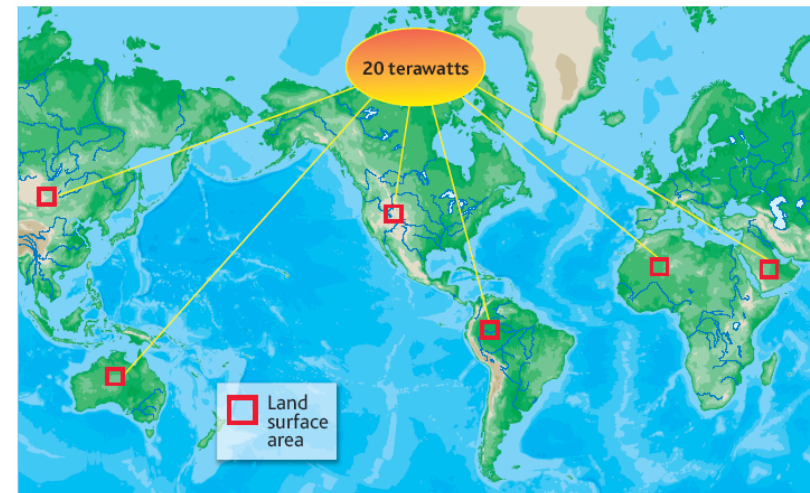
Global need. This map shows the amount of land needed to generate 20 TW with 10% efficient solar cells.
