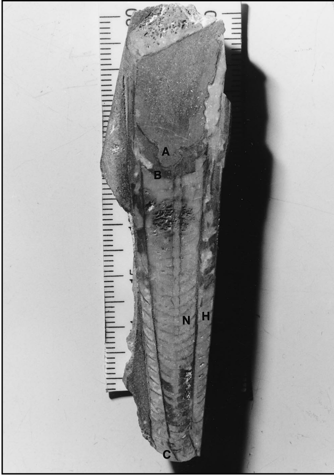
Figure 5. Partially imploded nautiloid, with imploded septa (A), and the first intact septum (B) (used for strength measurements) clearly visible. The unusual telescopic nesting phenomenon common in Graf samples (~60% of cut and polished specimens) also is observable in this sample. Note the outer, host shell (H) contains an inner, nested individual (N). In cases of nested samples, only the innermost shell, with no nested shells within it, can be used for septal strength measurements. Also note that the posterior tip of the inner nautiloid's phragmacone is broken (C), probably the result of high energy, violent impact with the host nautiloid's hardened cameral deposits. Specimen SUI83944A and SUI83944B. Scale is in centimeters (total length of nautiloid ~8 cm).
