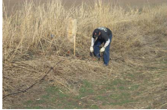
Figure 42. Connecting geophones still in place after January 2004 survey to cable laid down for March 2004 survey.
