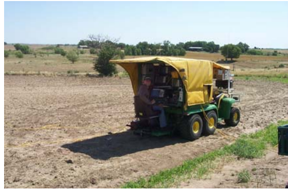
Figure 9. One of five Geode deployments (left) located in the center of each 48-station receiver line. The five Geode groupings were all connected to the Geometrics StrataVisor NZC seismic controller (right). Conducted from this John Deere Gator, seismic operations were all-weather and all-terrain. Here the Gator is configured for warm, dry conditions. Under wet or cold conditions an additional zip-on covering can be added to protect the operator and seismographs.
