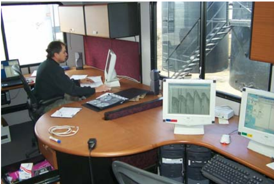
Figure 20. View from front of truck toward computer workstations (left); processing box (right) is climate controlled and mounted on truck frame with ride-controlled air suspension. A 12-kilowatt generator provides both 240-volt and 120-volt power. As data were acquired they were transmitted via Ethernet from the seismograph to the mobile processing center. Once data were transferred, preliminary processing was
