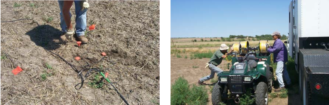
Figure 68. Geophones were planted (left) in a 0.3 m equilateral triangle centered on the DGPS-located station. Weatherproofed reinforced Ethernet cables stored on spools (right) connected the eleven 24-channel Geometrics Geodes to the NZC seismic controller. These cables were deployed using a custom cable handling system.
