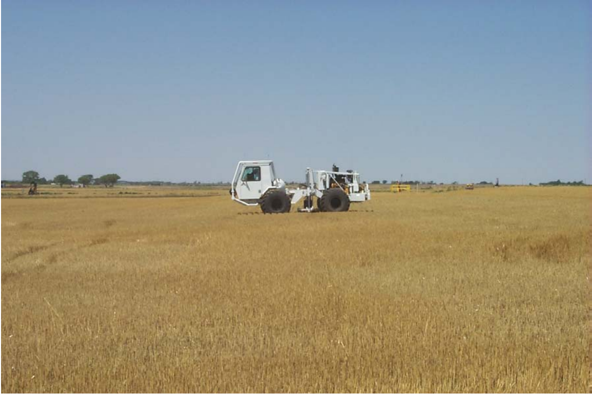
Figure 66. View looking west showing vibrator sweeping in the wheat stubble field surrounding the CO 2 injection well. Colliver #12 is visible on the horizon to the left of the vibrator in this picture. The CO 2 injector is enclosed in a yellow steel protection fence and can be seen immediately behind the vibrator, in the distance. Combines completed cutting wheat from this field just days before this picture was taken.
