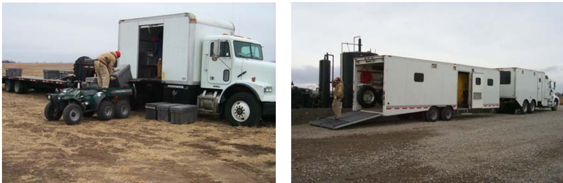
Figure 27. Two semi-trailers transport equipment to the field: (left) cables, phones, and vibrator, and (right) ATVs and seismograph.
