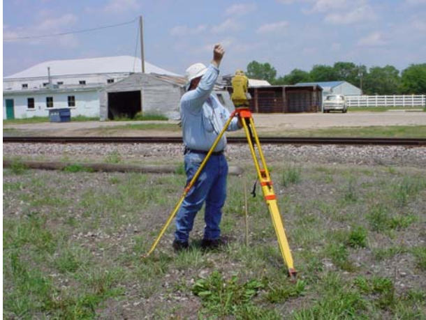
Figure 1. A theodolite (left) was used to define grids for high-resolution magnetic survey. David Laflen (left) is defining grids. A portable cesium gradiometer G858 (right) was used to measure the total component of the geomagnetic field. Jianghai Xia is performing the magnetic survey.
