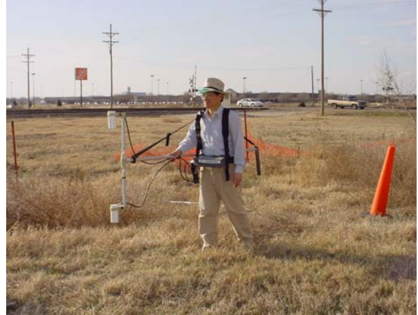
Figure 1. A theodolite (left) was used to define grids for high-resolution magnetic survey. David Laflen (left) is defining grids. A portable cesium gradiometer G858 (right) was used to measure the total component of the geomagnetic field. Jianghai Xia is performing the magnetic survey.
