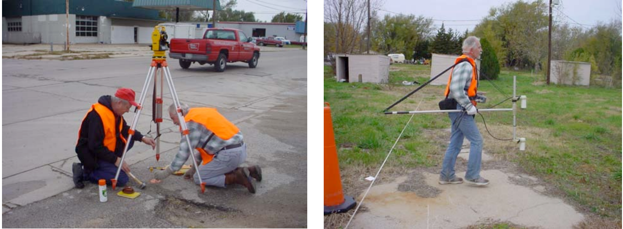
Figure 1. A theodolite (left) was used to define grids for high-resolution magnetic survey. James Kelly and Ron Wilson was setting up the theodolite. A portable cesium gradiometer G858 (right) was used to measure the total component of the geomagnetic field. Ron Wilson was performing the magnetic survey.
