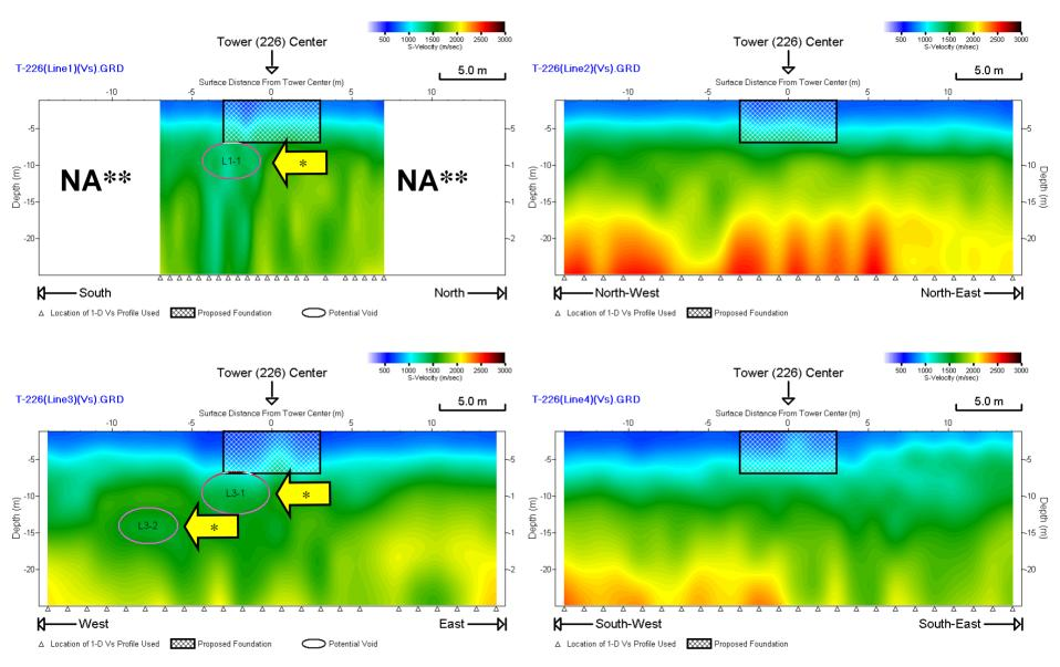
\*Potential void (see separate text file for coordinates), \*\*A shorter receiver spacing of 2 ft was used due to terrain condition (steep drop off).
