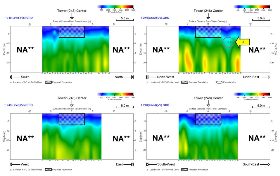
\*\*Data not acquired due to terrain condition (shorter receiver spacing of 2 ft used), \*Potential void (see separate text file for coordinates)
