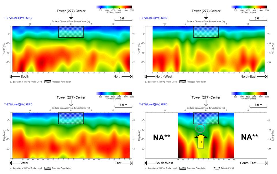
\*Potential void (see separate text file for coordinates), \*\*Data not acquired due to terrain condition (steep drop off)
