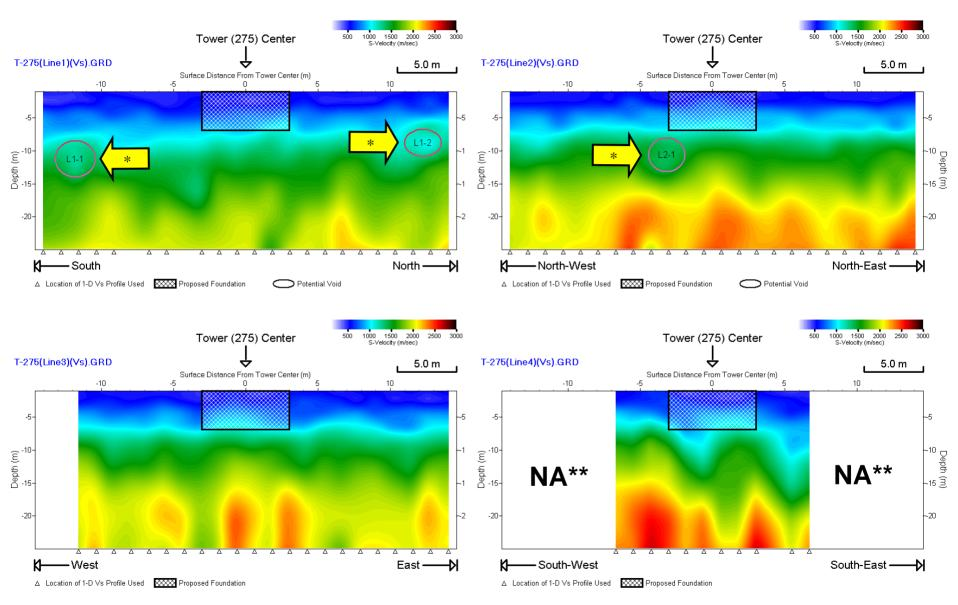
\*Potential void (see separate text file for coordinates), \*\*Data not acquired due to terrain condition
