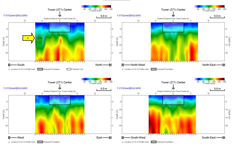
\*\*A shorter receiver spacing (2 ft) was used for all four (4) lines due to terrain condition. \* Potential void (see separate text file for coordinates)
