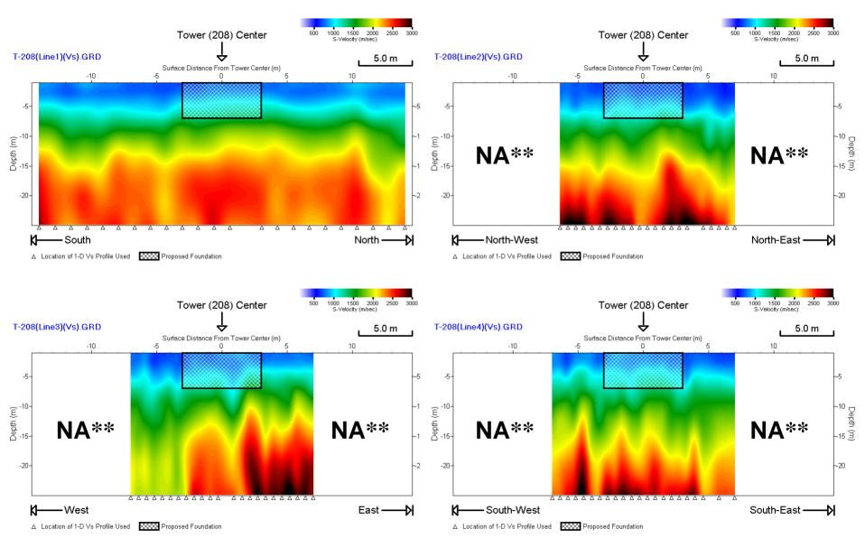
\*\*All East-West lines (2, 3, and 4) used a shorter receiver spacing of 2 ft due to terrain condition (steep drop off).
