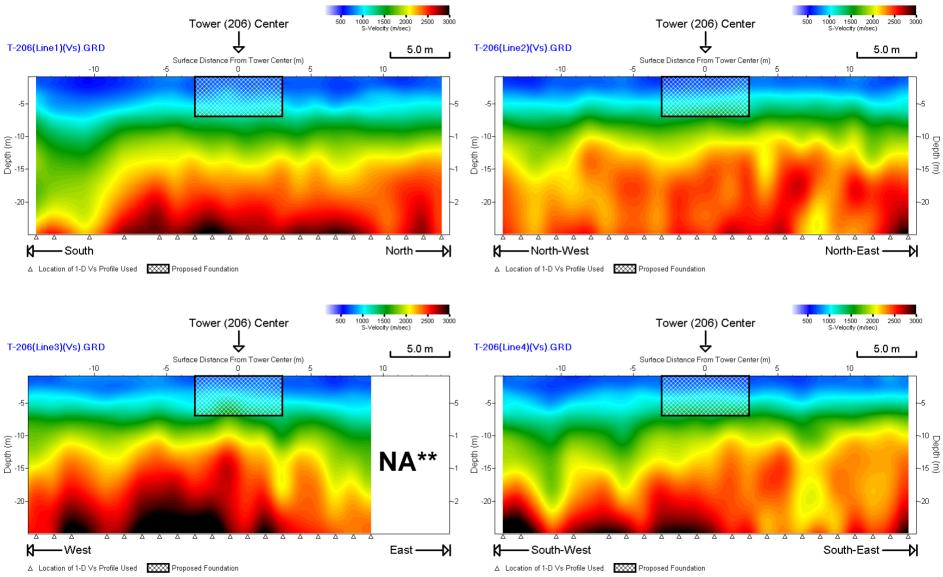
\*Line 4 shifted to north by 6 stations (=24ft) from the planned position (12 stations south of tower center) due to terrain condition \*\*Data not acquired due to terrain condition (steep drop off)
