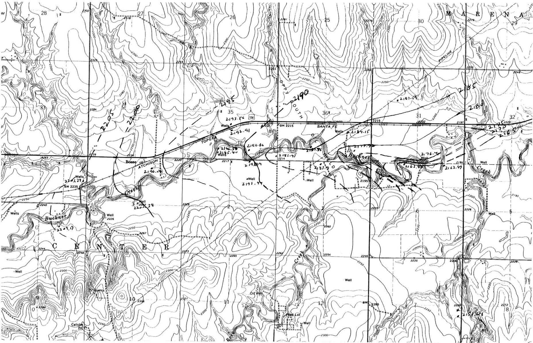
Figure 2. Configuration of the water-table surface in the alluvial aquifer of Buckner Creek from water-level measurements made in March 2000.
