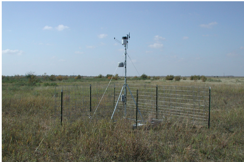
Figure 12 – Weather station at Ashland viewed from the south (a) and east (b). Tipping-bucket rain gage is on the right end of cross bar in photograph (a), while wind-speed and direction sensors are on left end of same cross bar. Solar radiation sensor (pyranometer) is on slanted arm extending outward to the south (left) near top of weather station in photograph (b). Relative humidity and temperature sensors are in radiation shield at an elevation of two meters above lsf. Barometer is inside datalogger housing located on main pole below point where support legs connect to main pole. Dave Arnold home is in the distance in the center right of photograph (a).
