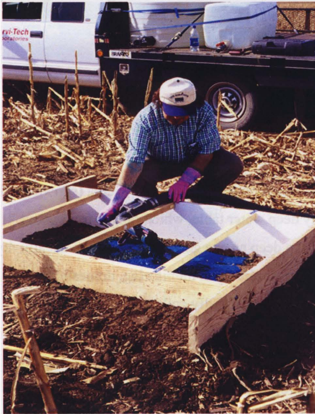
Figure 3. Wooden rectangular frame for flooding the site with dye solution.
