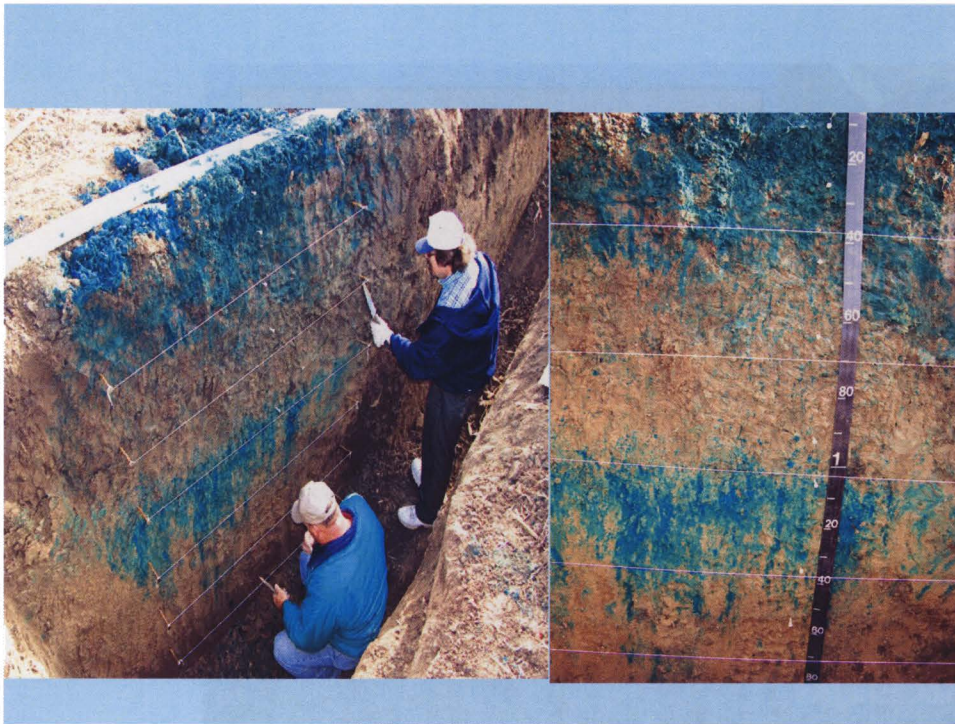
Figure 12. Uniform finger front from brilliant-blue dye-tracer experiment at site R8. The right-hand-side image shows in more detail the dye moving through the inter-soil block structure spaces of the Bt horizon and accumulating below that blocky layer into numerous fingers.
