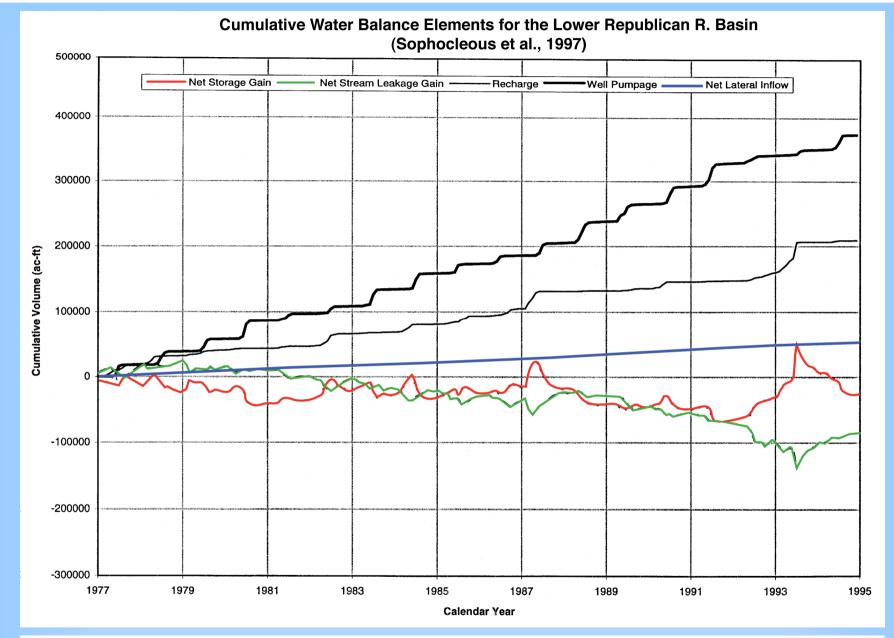
Net GW Storage Gain = GW Storage Accumulation – GW Storage Depletion Net Stream-leakage Gain = Baseflow – Stream-leakage loss
