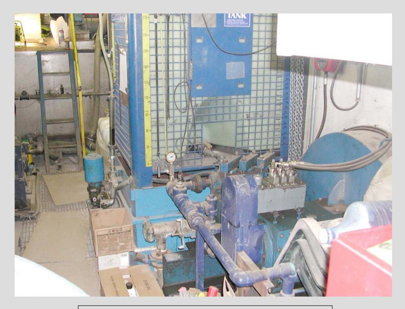
Tri-plex pump and crosslinker storage
