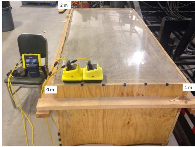
Figure 4.1: Photo of the sandbox used for the controlled GPR experiments. GPR lines were run parallel to the long axis of the box.
