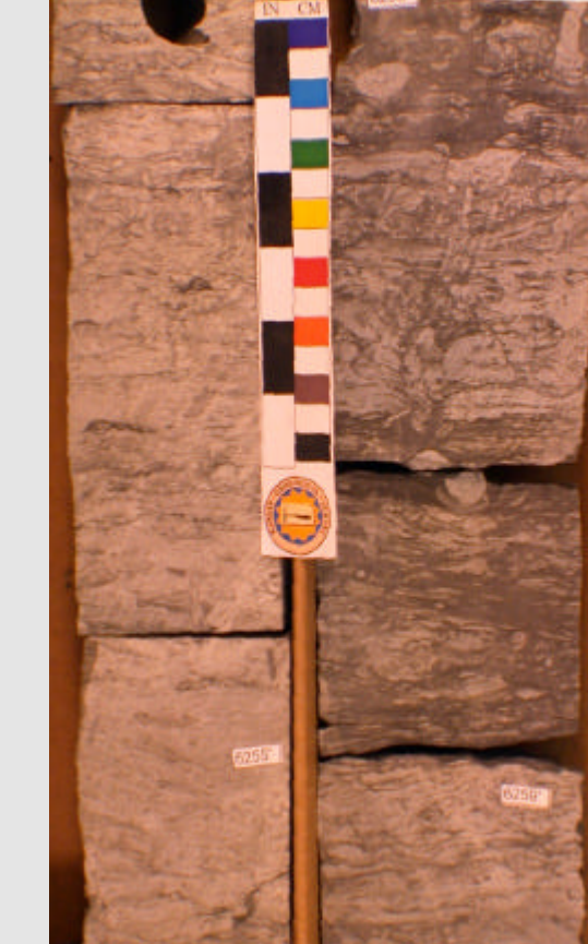
(Kniffen A-2, 6254'-6259') Light gray, fine to very fine sandstone, calcareous, glauconitic, interlaminated with dark gray shale, highly horizontal and vertically burrowed.
