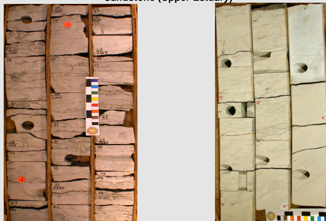
(Breeding Gas Unit F-1, 5257.7'-5264.7') Light gray, fine sandstone, often glauconitic, slightly to non calcareous, well to moderate sorted; mud drapes, flaser and wavy bedding; occasionally starved ripples. Some horizontal burrowing.
