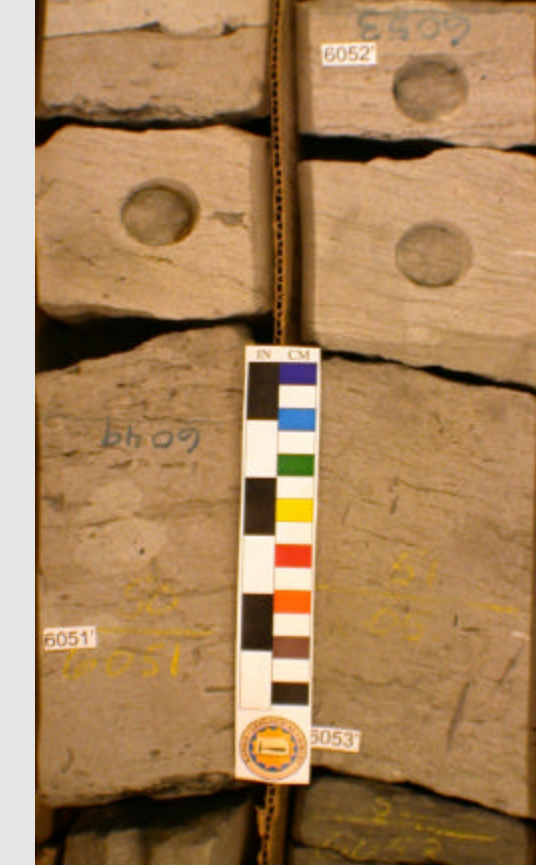
(Neill A-1, 6050'-6053') Light gray, fine to medium sandstone, glauconitic, calcareous, fossiliferous, moderate to well sorted; common low-angle cross beds. Some vertical burrows.
