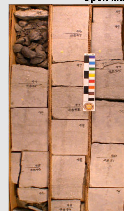
(Longwood Gas Unit 2, 4844.5'-4852') Light gray or brown, crinoidal packstone to wackestone with fossil fragments (brachiopods, bivalves, bryozoans and rare corals).
