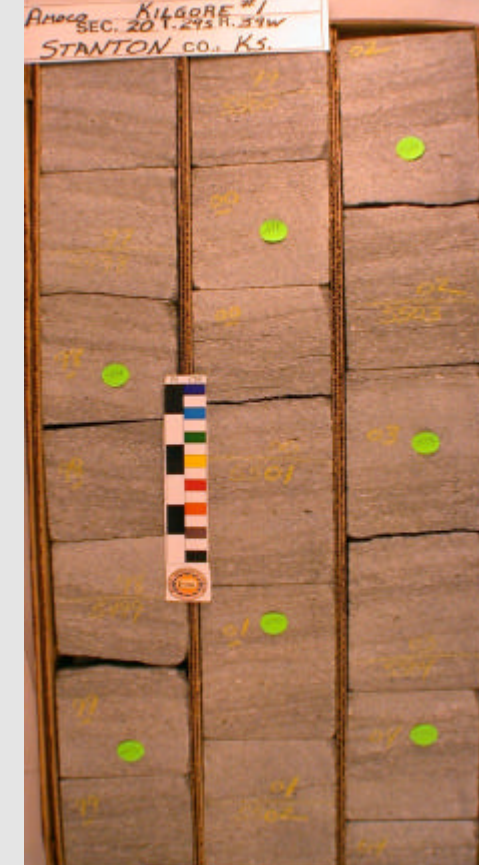
(Grace Kilgore 1, 5492'-5504') Light gray, coarse to medium sandstone, glauconitic, calcareous, fossiliferous, moderate to poorly sorted, with high-angle planar parallel cross beds and subhorizontal parallel laminations.
