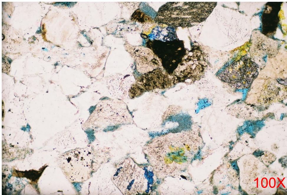
Figure 4.5.7. Example Mesaverde thin-section for Type IV porosity. Porosity consists almost entirely of sparse, poorly connected, clay-filled intergranular microporosity. Quartz cement is prominent, ferroan calcite is sparse. Pore-filling clay cement causes elevated S_{wi} , reduced relative permeability, and increased P_c entry pressure. Williams PA 424, 4686.4', Rock type 15286, \phi = 7.9\% , GD = 2.65 g/cc, K_a = 0.211 mD.
