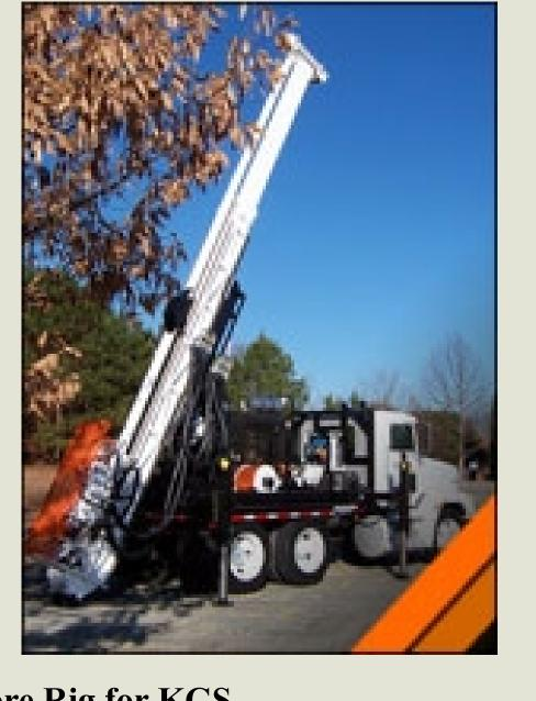
New Core Rig for KGS Longvear-LF90D Hydraulic Diamond Core Drill
