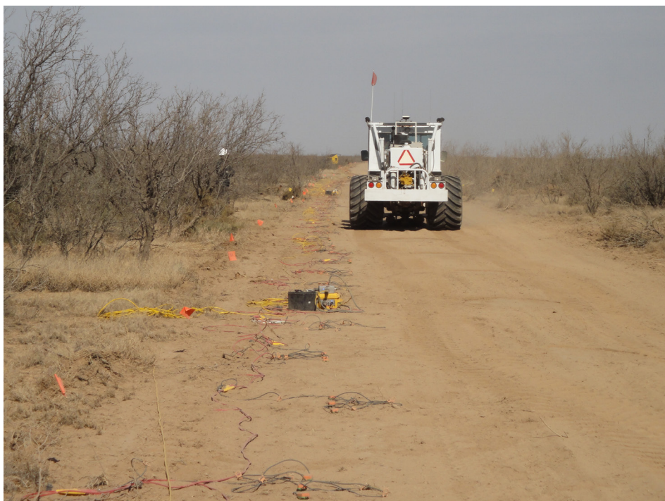
Figure 7—Geophones connected to seismographs (yellow boxes located next to black batteries) during an active seismic survey.
