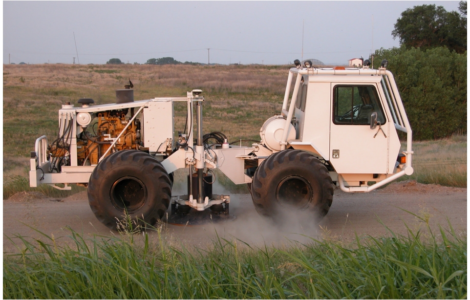
Figure 1—The KGS uses a commercial seismic vehicle, the IVI minivib (shown here in Russell County), to drive a weight into the ground with a series of low-power impacts that produce seismic waves, which are recorded and analyzed.
