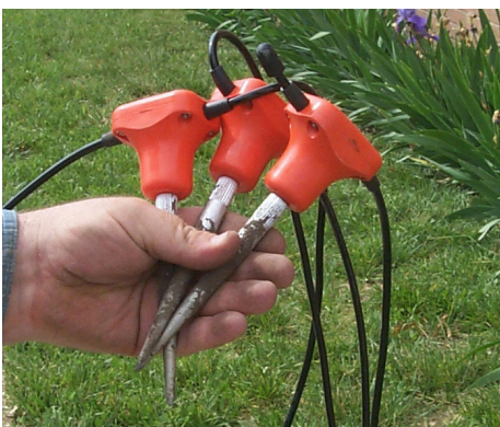
Figure 5—Geophones used by the KGS for active seismic surveys.
