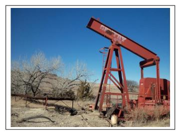
The Hadley well # 12 located in the SW NW SW NE has an open hole with rods laid out in doubles. **API # 15-051-02234-00-01.**
