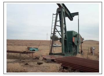
**Photos taken January 10, 2023** The Henry Mai well # 1 located in the SW SW SW SE has an open hole with rods stacked in doubles. **API # 15-051-02165-00-00**.
