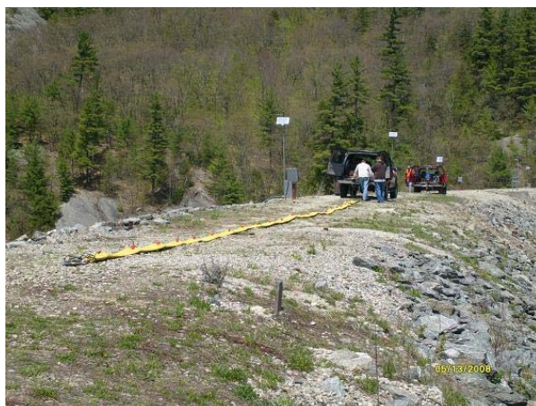
Figure 3. View to the north from the dam crest. Seismic data were acquired with a towed array and both a near-offset hammer and a far-offset weight-drop source.
